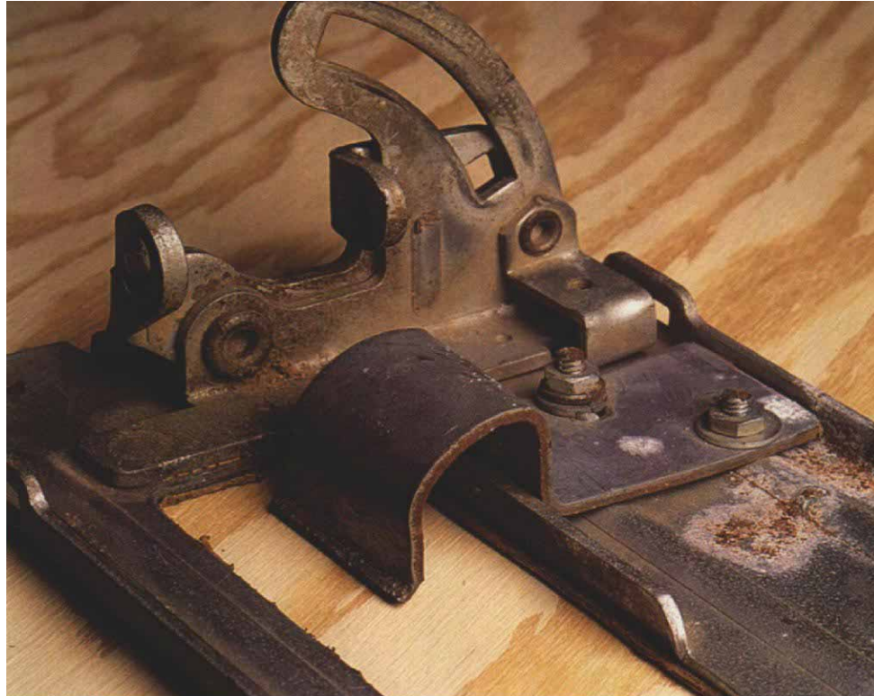
The saw flange. This homemade metal flange bolts to a circular saw's baseplate. The edge of the flange rides along the cutline to hold the wood fibers in place. Placed properly, it won't interfere with the operation of the blade guard.
