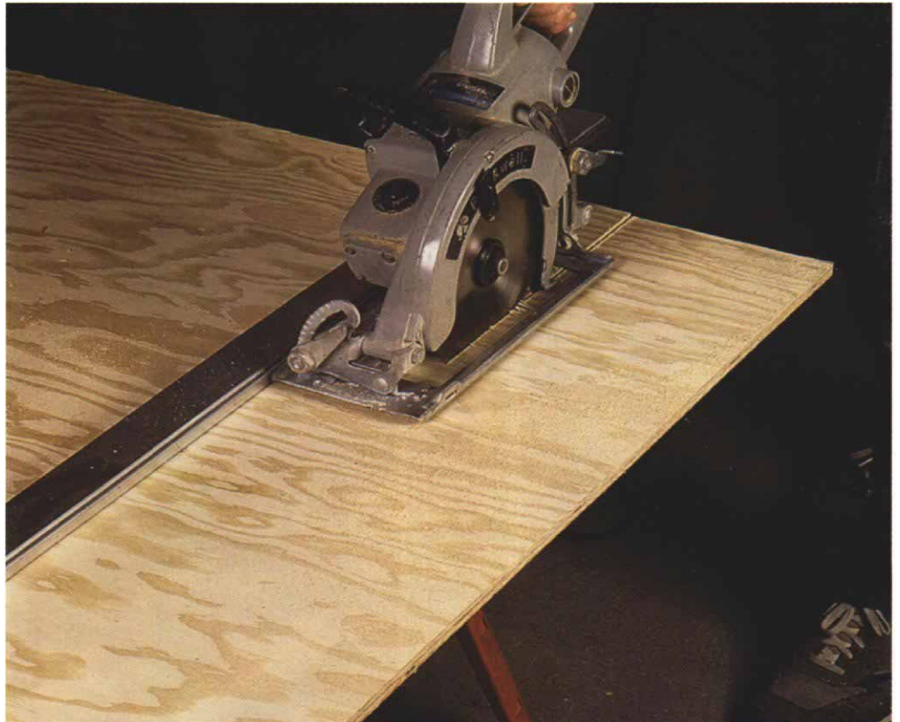
A guide to straight cuts. This cutting guide includes built-in clamps that set easily to grip panel stock. The 50-in. length of the tool means it can guide cuts across the width of a plywood sheet.
